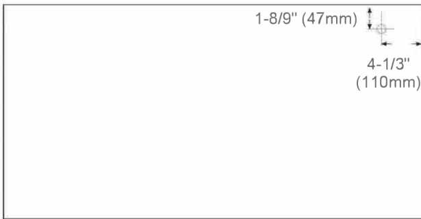
Back of Cabinet - Wire Access Location
