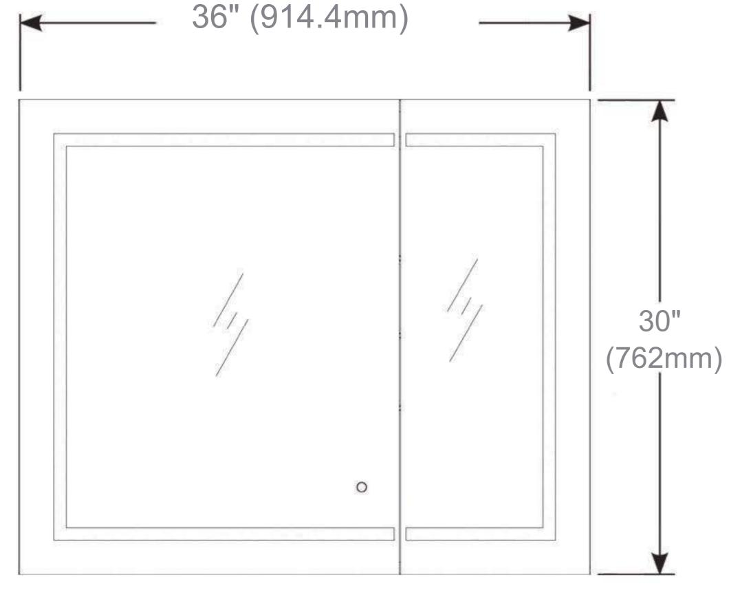
Rough-in Depth Minimum 4" (102 mm) Required (749mm)
