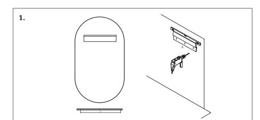
1. Before your installation, measure the distance A of bracket, and drill holes in the marked positions by using a suitable tool.
