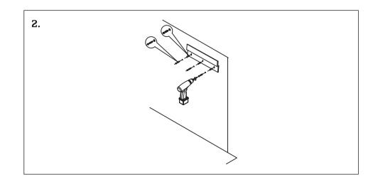
2. Insert the wall plugs on the surface of the wall. After that, fasten the supplied screws into wall plugs.
