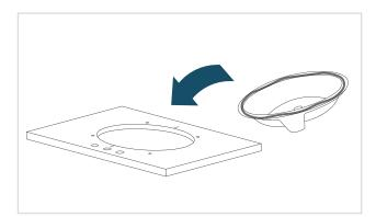
**STEP 3 -** FLIP & SET IN PLACE Carefully flip the sink basin over and place it so the guide lines match up in both locations.
