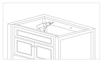
**STEP 6 -** ATTACH BASE CABINET TO WALL Place cabinet in desired location and detmine where the wall studs are. Using drywall screws, attach the cabinet to the wall by screwing into the wall studs.
