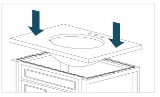
**STEP 8 -** SET COUNTERTOP IN PLACE Carefully place the countertop, with the sink attached, onto the cabinet and press down firmly. Wipe away and excess silicone immediately.
