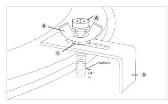
**STEP 5 -** ATTACH UNDERMOUNT CLIPS Please tighten Bolt (A) into wing nut (B) slide on washer (C) and guide through Under-mount clip (D) opening into threaded bolt hole in the countertop. ONLY-Hand Tighten Bolt (A) to a depth of about 1/4" below countertop surface. Then secure the Sink with the under-mount clip (D) by Tightening wing nut (B) only
