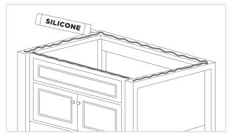
**STEP 7 -** PREPARE BASE CABINET Using a caulking gun, apply silicone around the top of the base cabinet.
