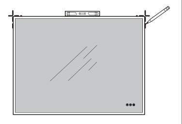
**SUPPORT LOCATION** Measure the center of the holes and mark the drilling locations ensure marking are leveled.
