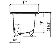
\*8" C.C. waste/overflow to drain Top center of overflow to floor 19 1/2"
