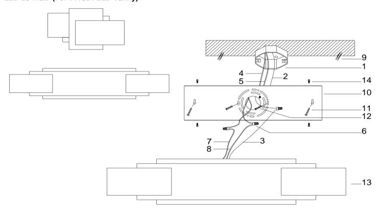
1.OUTLET BOX(not included) 2.SUPPLY GROUND WIRE(not included) 3.FIXTURE GROUND WIRE 4.BLACK SUPPLY WIRE(not included) 5.WHITE SUPPLY WIRE(not included) 6.WIRE CONNECTORS 7.RIBBED(or WHITE) FIXTURE LEAD WIRE
