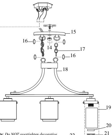
**Note**: *Do NOT overtighten decorative* screws (23) that go through rubber washers (22) and clear glass shades (24) as alabaster glass shades (19) may crack or break.
