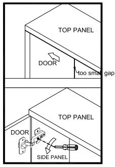
Turn the screw counterclockwise a little as shown to make the gap big.
