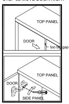
Turn the screw clockwise a little as shown to make the gap small.
