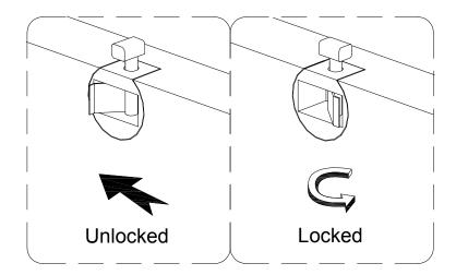
Reference the images above any time the instructions state "lock the hardware". Note: Be sure to check all hardware is locked when completed.
