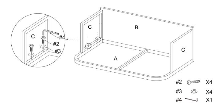
Step 3. Attach front panel (part D) to assembled unit (parts B & C) using long bolts (part #2), flat washers (part #3) and allen wrench (part #4).
