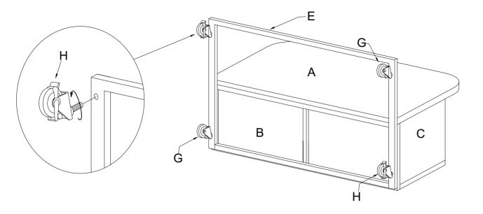
Step 6. Carefully turn unit upright. Attach divider (part F) to bottom frame (part E) using short bolts (part #1), flat washers (part #3) and allen wrench (part #4).
