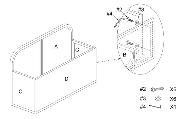
Step 4. Attach bottom frame (part E) to assembled unit (parts B & C) using long bolts (part #2), flat washers (part #3) and allen wrench (part #4).
