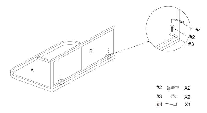
Step 2. Attach side panels (part C) to back panel (part A) using long bolts (part #2), flat washers (part #3) and allen wrench (part #4).
