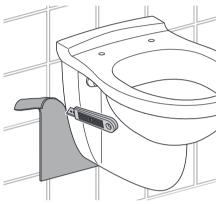
**10** Seal gap around bowl with waterproof sealant.
