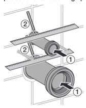
Place discharge pipe with gasket into waste outlet of bowl. Also place flush pipe with fin gasket into inlet of bowl. Then mark a second line on both pipes.
