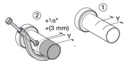
Bevel the sharp edges as shown to assure a smooth insertion into the pipe hubs in the wall.
