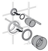
Insert discharge pipe into the pipe hub in the wall. Place a straight edge flush against the wall and mark a line on the pipe. Fit finned rubber seal onto flush pipe. Repeat same procedure for discharge pipe.
