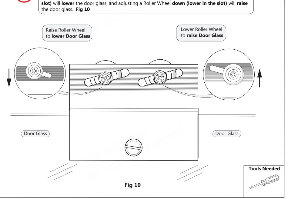
The **Roller Wheels (#12)** can be adjusted to better align the vertical edges of the **Door Glass** with the **Wall Profiles** if needed, to prevent leaks. In order to adjust either side of either door up or down, remove that door from the **Guide Rail (#08).** Use a helper and be careful to
