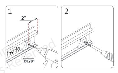
**Fig 3** (Bottom Guide Rail shown)
