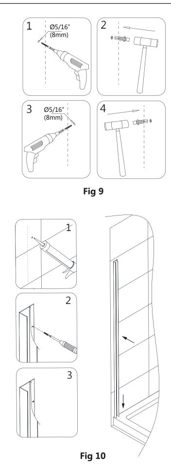
10. Apply a bead of silicone to the back of the Wall Profiles (#01) and the screw holes where the Wall Profiles (#01) will be installed. Attach the Wall Profiles (#01) to the wall using the ST4.2 x 40 Truss Head Screws (#05). Repeat this process for the opposite wall profile. (Fig 10)
