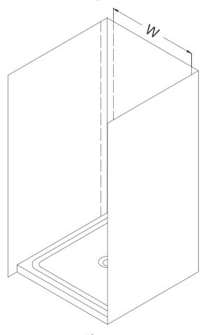
3. The **Back Panel (09)** has **3-1/8**" flange on both sides and has to be cut equally from both sides if necessary.
