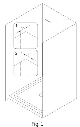
2. Measure the back wall of the shower between the vertical lines you marked in <a href="Step 1">Step 1</a>. This distance is marked as "W".
