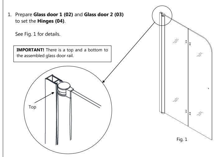
First, attach the Hinges (04) to Glass door 1 (02), then attach Glass door 2 (03) to the Hinges (04). Be sure to install the rubber gaskets that come with the hinges to protect the glass from contact with the metal.
