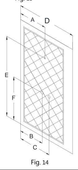
12. Drill the holes for the fixtures in the **Side panel (01)** using the proper diameter saw bit or a handheld jig saw.
