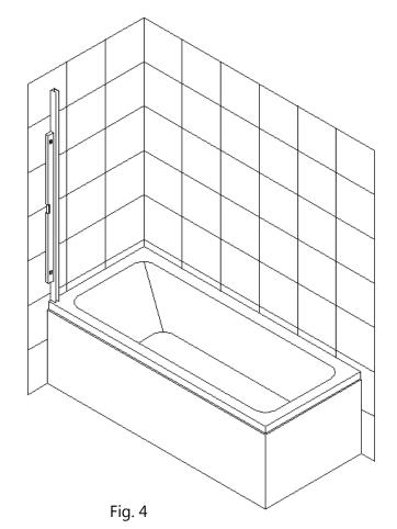
4. Mark the drill holes on the wall through the predrilled holes in the Wall profile (01). Now drill holes in the wall using a Ø5/16 drill bit and insert the Wall anchors (05). Apply silicone along the Wall profile (01) and around the holes. Fasten the Wall profile (01) to the wall with the Big head Screw ST4.2×40 (06).
