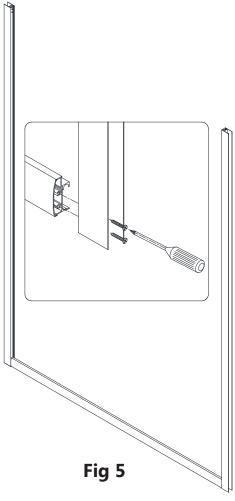
**<u>TIP</u>**: For ease of assembly, add some liquid soap, wax or lubricant to the screws prior to attaching the glass profiles to the guide rails. Use a low setting on your power drill to prevent stripping the screws.
