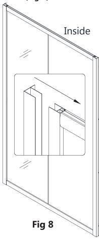
**9.** Move the assembled frame into the designated position on the shower base\*, bathtub or threshold (depending on your installation), and push the Wall Profiles (#02) tight to the walls to compensate for any out-of-plumb conditions.
