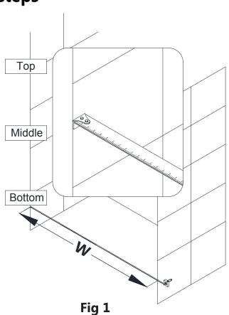
**2.** Subtract 3-3/8" from your finished opening (W) to determine the finished cut length for the Top and Bottom Guide Rails (#03). Cut the Top and Bottom Guide Rails (#03) to the finished cut length "D". **Cut from the door end only,** (which is the end farthest from the glass holder hole) and cut each rail to the same length from the same end. (Fig 2 and Fig 3)
