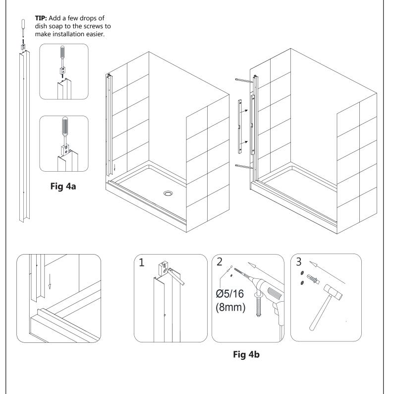
**5.** Apply silicone to the back of the **Wall Profile (#01)** and place it back into position on the wall. Attach the **Upper Guide Rail Connector (#07)** using two each of the **ST4.2** x **40 Countersunk Flathead Screws (#10)**. Attach two of the **Wall Profile Bumpers (#04)** using the **ST4.2** x **10 screws (#11)** and cover the holes with the decorative caps.
