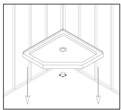
Lower the base over the drain pipe and set it into place against the studs.
