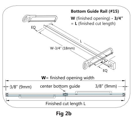
**3.** Place the **Bottom Guide Rail (#15)** onto the threshold in the desired position. Use a tape measure to align it evenly with the front edge of the threshold and mark its position on the threshold.
