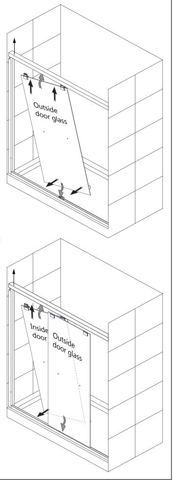
**14.** To compensate for minor out-of-plumb conditions (up to 3/8"): After both doors are installed, use the **Allen Wrench (#14)** to make minor adjustments with the **Roller Assemblies (#06)** as necessary.
