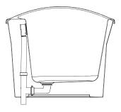
Standard drainpipe and overflow compatible with center drain freestanding bathtub models: BTMO6032WFXXC00, BTMO6636WFXXC00 (Montego), BTCA6032WFXXC00, BTCA6636WFXXC00 (Caspian)
