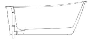
Standard drainpipe and overflow compatible with end-drain freestanding bathtub models: BTSC6032WFXXF00 (Seneca)
