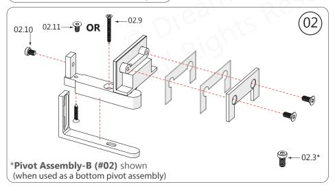
The Pivot Assemblies are paired and either one can be used as the top or bottom pivot depending on the handing of the door installation.
