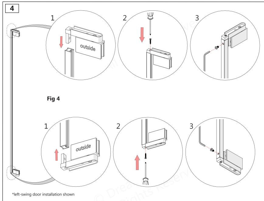
The Glass Profile for Pivot Side (#04) is the shorter of the two Glass Profiles and has an additional pair of holes at each end. These extra holes are not present in the Glass Profile (#05) that is used for the strike-side.
