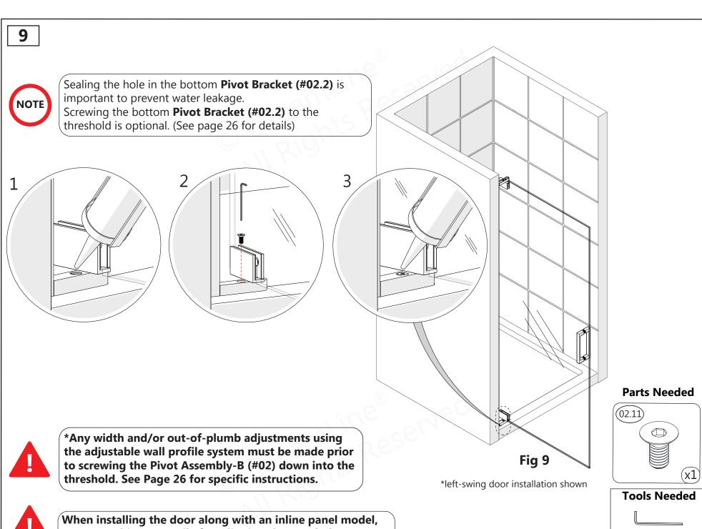
postpone this step until after aligning the panel glass.
