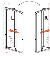
This door is reversible for right- or left-hinge door installation. The left-hinge door installation is shown throughout this manual. For the right-hinge door installation, simply begin on the opposite wall and reverse the orientation of the installation steps shown.
