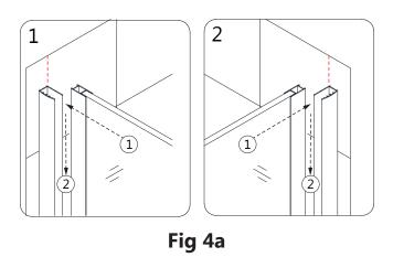
**5.** Examine the **Pivot Bars (#05)** and notice that there are holes for the top and bottom pivot assemblies on one end. Attach the top and bottom Pivot Bars (#05) (with the pivot holes on the correct side for the swing of the door) through the holes in the Panel Glass (#03).
