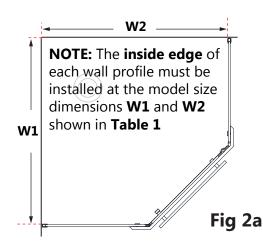
Table 1 - Enclosure assembly measurements
