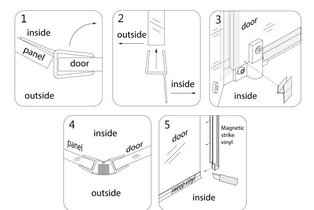
**Fig 8**Left-hand door installation shown
