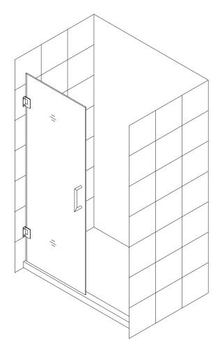
NOTE: The Unidoor hinge is factory set to over close 8°. The following procedure is recommended to ensure proper alignment of the panel glass and the door glass.
