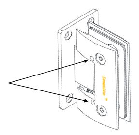
**5a.** Make sure the door glass is plumb and the edge of the hinge is installed flush with the glass edge. Center the hinge in the glass notch and tighten the faceplate screws **(Fig 5a)**. Be careful not to scratch the finished surfaces of the hinge during installation.
