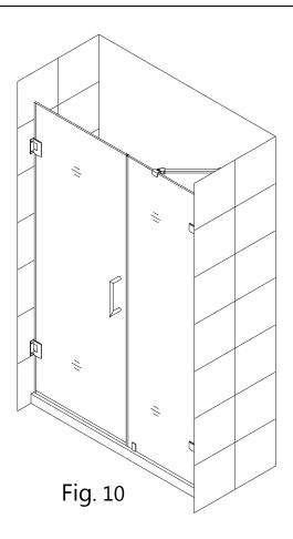
Apply good quality mildew-resistant silicone along the connection of the Stationary glass (11) with the walls and the threshold.
