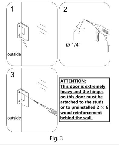
**TIP:** The PVC hinge spacer can also be used as a template to assist with marking the hinge mounting holes.
