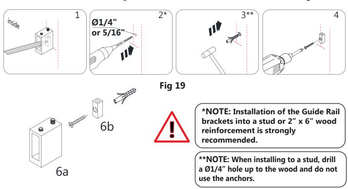
20. Re-attach the Guide Rail (#04) to the Stationary Glass (#02) and attach the Guide Rail Brackets (#06). (Fig 20)
