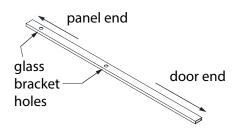
**NOTE:** Use a metal file to remove any burrs from the cut end of the Guide Rail (#04).
