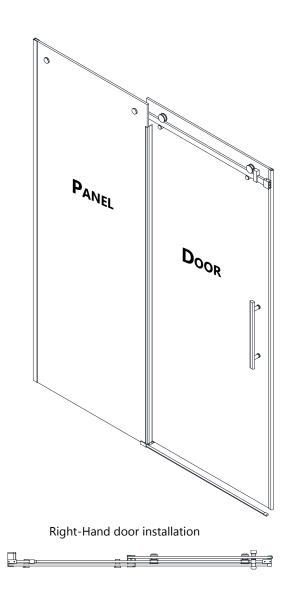
**NOTE:** This door is reversible for right or left-hand door installation. The right-hand door installation is shown as an example throughout this manual. For the left-hand door installation, simply begin on the opposite wall and reverse the orientation of the steps shown.
