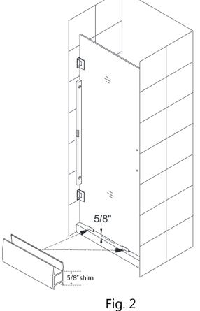
**3.** Hold the door in place and mark the drill holes for both **Hinges (05)** on the wall. Set the door aside and use a Ø 1/4" drill bit to drill holes up to the stud. Drill 1/8" pilot holes into the stud if necessary.
