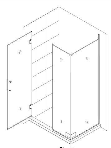
NOTE: The next step involves careful handling of the glass panels that were just temporarily fixed together to determine a custom fit measurement unique to your installation. It is essential that two installers be used along with responsive communication.
