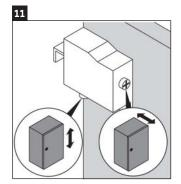
Screw two set screws until desired leveling of the vanity has been reached.
