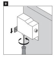
Using a screwdriver adjust the vanity mounting hinge system counter-clockwise.
