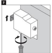
Using a screwdriver, adjust the vanity mounting hinge system clockwise.
