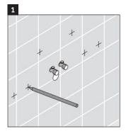
Reference the washbasin specification to establish the position of mounting bolts, mark the holes to be drilled for the anchors.
