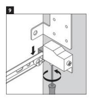
Using a screwdriver, adjust the vanity mounting hinge system clockwise.
