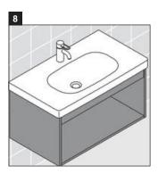
Slide the vanity under the washbasin. Tighten mounting unts with a wrench until the washbasin is stable.
