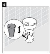
Turn bottom screw counter -clockwise to adjust unit up and down.
