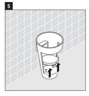
Lift the unit up and onto the mounting screws.
