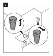
Check the screws which allow adjsutment of the unit. The top screw will adjust front to back and the bottom screw will adjust up and down.
