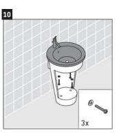
Using three screws and three washers secure the washbasin to the vanity.
