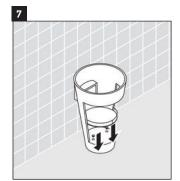
Slide the unit down onto the mounting screws.
