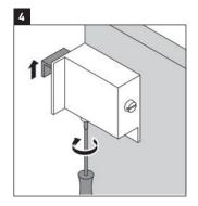
Using a screwdriver, adjust the vanity mounting hinge clockwise.
