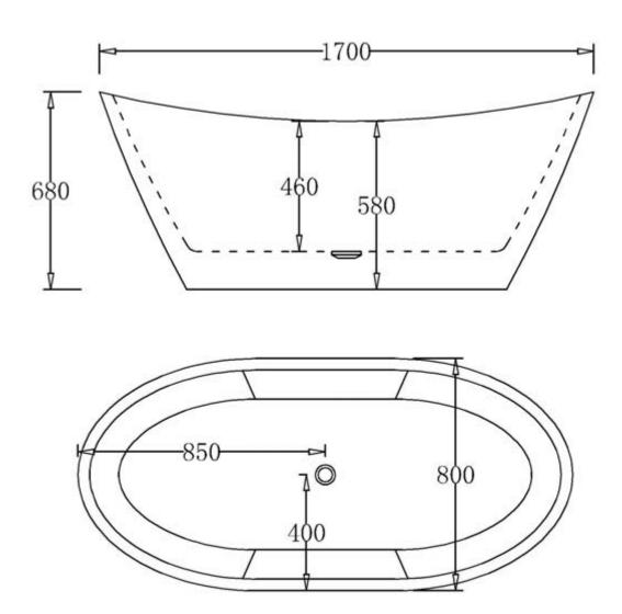
Note: Measurements are in millimeter and can vary by ±15 millimeter
