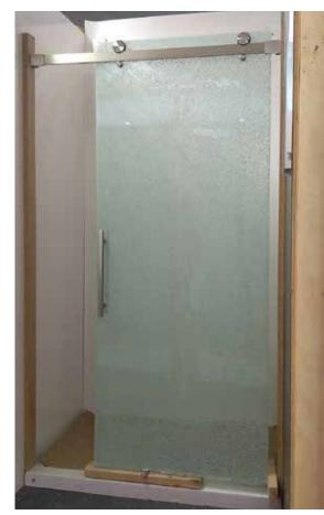
Shattered glass maintains structure with S.R.T. film
