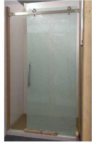
Shattered glass maintains structure with S.R.T. film
