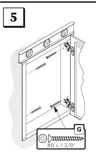
Level, then secure the medicine cabinet with the screws  $(\mathbf{G})$ through the mounting holes into the framing studs.
