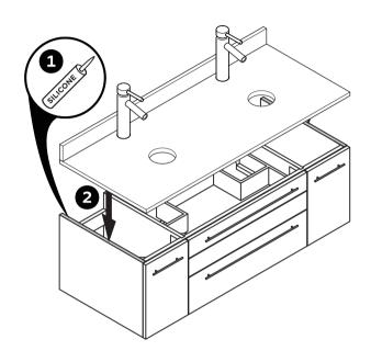
Apply a bead of silicone on the top of counter top and the bottom of the sinks. Connect sinks to the counter top.
