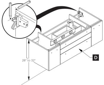
Apply a bid of silicone and hang the cabinet (D) on the brackets (E).
