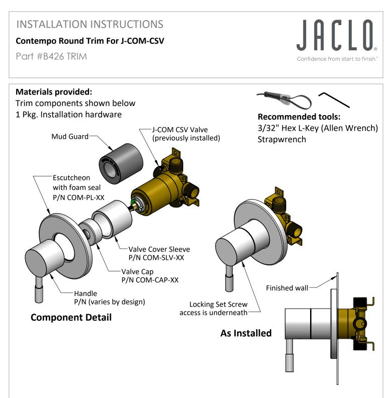
**Step 1:** Tap (or strike lightly to break free) the black Mud Guard, remove and dispose.
