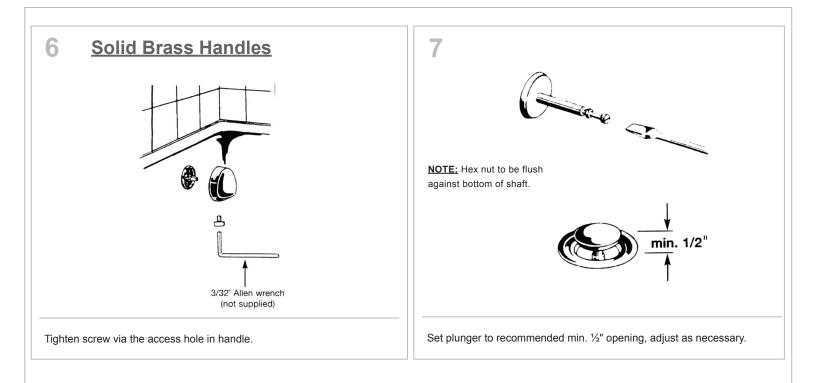
To operate drain, simply turn handle 1/8 turn (clockwise opens, counter-clockwise closes).
