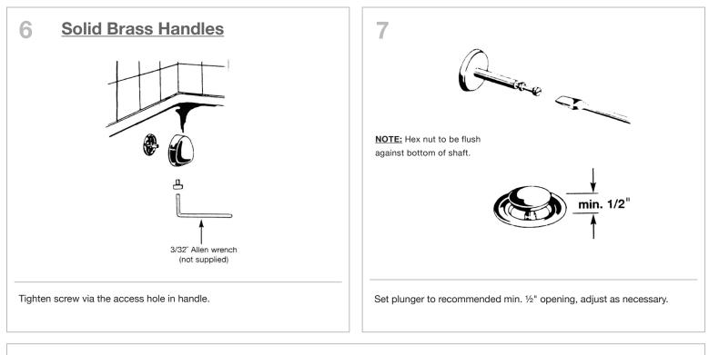
To operate drain, simply turn handle 1/8 turn (clockwise opens, counter-clockwise closes).
