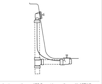
For solvent connection use ABS Cement in compliance with ASTM D 2564-88 ONLY.
