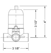
WATER ON/OFF AND TEMPERATURE CONTROL ROTATE LEVER FULL ON
