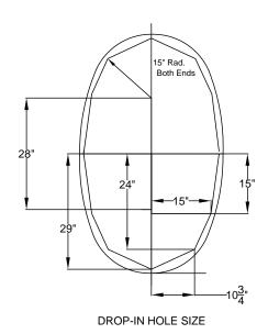
Note: The pump extends approximately 1" past the end radius of the bath. This requires angling the bath into the drop-in hole.
