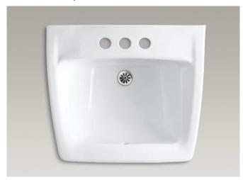
The Chesapeake wall-mount lavatory provides outstanding performance ideal for commercial settings. You can count on durable vitreous china construction to maintain its hard, nonporous finish for a remarkably clean, sanitary lavatory and years of reliability. This ledge-back sink includes wall hanger, and also features drillings for a concealed arm carrier and a faucet with 4" centers.
