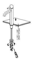
Install the faucet through the 1-3/8" predrilled hole in the countertop. Attach rubber washer (4A), metal washer (4B), mounting nut (4C), and mounting screws (4D) on the threaded mounting pipe. Tighten the mounting nut (4C) until snug. Tighten screws (4D) on the mounting nut (4C) with a Phillips head screwdriver until snug.
