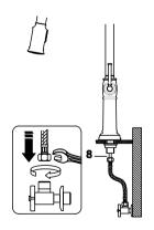
Connect waterlines (8) to angle stops. Tighten both ends of waterlines with a wrench until snug. Turn on hot and cold angle stops and check for leaks.
