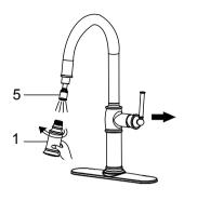
Remove spray head (1) from spray hose (5). Hold tip of spray hose (5). Turn faucet on and let the water run for 60 seconds to flush any debris.
