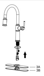
For three-hole installation: Deck plate (3A), base plate (3B), and silicone sealant (optional) are required.
