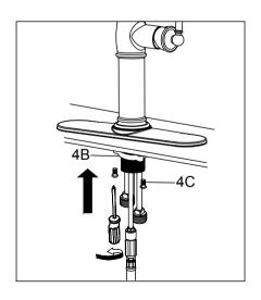
Adjust direction of faucet body (2) so that handle is on right side of faucet. Tighten mounting nut (4B) until snug. Tighten mounting screws (4C) to nut with a Phillips screwdriver until snug.
