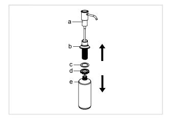
Install dispenser base (b) with washer attached into the hole in the countertop. Re-install washer (c) and mounting nut (d) on the dispenser base (b) from underneat countertop. Tighten mounting nut (d) by hand.
