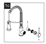
This indicates that the cartridge is damaged. Turn off the water supply, remove the handle and replace the cartridge (1).
