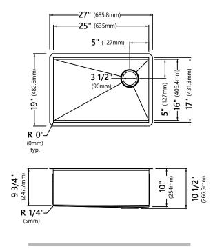
Model #: KWU110-27 & KWU110-27/PGM Sink Dimensions: 27" x 19" x 10" Min Cabinet Size: 30"
