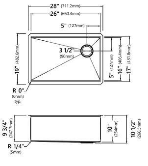
Model #: KWU110-28 Sink Dimensions: 28" x 19" x 10" Min Cabinet Size: 30"
