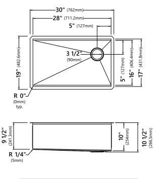
Model #: KWU110-30 Sink Dimensions: 30" x 19" x 10" Min Cabinet Size: 33"
