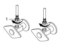
Thread the nut (1) on the supply line onto the outlet of the water supply valve and tighten with a wrench. Do not overtighten.
