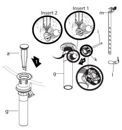
Insert waste stopper (a) into drain flange. Remove extender rod (m) and clip (l) from drain off pole (i). Reomve nut (k). Insert drain off pole (i) into drain pole opening of tailpipe (g). See insert 1. Secure nut (k) to drain off pole opening of tailpipe (g).
