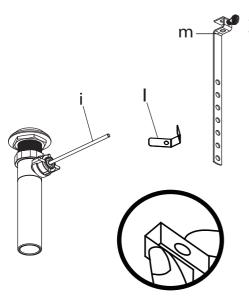
Attach drain off pole (i) to extender rod (m) with clip (I).
