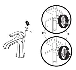
Loosen thumb screw (n) on extender rod (m). Push down on lift rod (o) until stopper is in open position. Retighten thumb screw (n).
