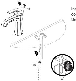
Insert lift rod (o) through spout and connect with extender rod (m). Tighten thumb screw (n).
