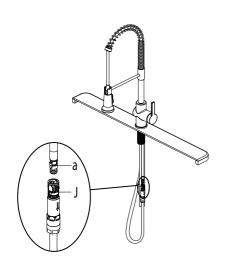
Push the quick connector (J) firmly upward and attach it to the receiving block (a). Pull down moderately to ensure the connection has been made.
