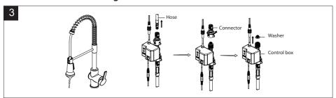
a.This could indicate that the washer in the control box is dirty or damaged. Remove the hose and unscrew the connector. Take out the washer from the control box. Clear the washer or replace the washer. Reassemble the
