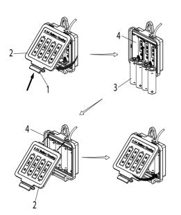
To open the battery housing, squeeze the tabs (1) on the cover (2), then remove the cover (2). Install the four AA batteries (3) included by matching the positive (+) and Negative (-) ends on the battery (3) to the (+) and (-) markings in the battery pack (4). The negative ends of the battery (3) should always connect to the spring end of the battery slots in the battery pack (4). Reinstall the battery pack cover (2) by pushing up and snapping into place.
