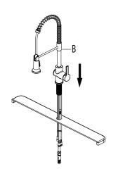
Shut off the water supply. Insert faucet body (B) through the hole inthe sink.
