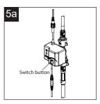
If you want to use the faucet without the sensor feature, you can loose the switch button completely with a coin counterclockwise. At this time, you can use the sensor faucet as the use of the common faucet.
