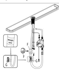
Install the weight clip (G) at the point of the hose marking "weight here". Insert the weight (F) onto the weight clip (G) by sliding it down onto the weight clip (G).
