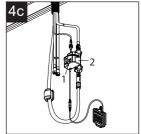
Check whether the switch button (1) is tighten, if it is loose, tight the switch button (1) completely with a coin clockwise. If the switch button (1) is tighten, this indicates that the control box (2) is damaged. Call customer service to request a replacement control box. Replace the old control box with the new control box.
