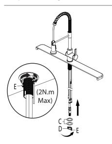
Secure the faucet (B) to the countertop using the washers (C) and mounting nut (D) provided. Hand tighten the nut (D) onto the faucet assembly. Lock the nut (D) into position by tightening the screws (E) with a phillips screwdriver. Do not overtighten.
