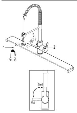
Flushing and checking for leaks: After the installation is complete, unscrew and remove the spray head in order to flush the line. Turn on the water supply and allow both hot and cold water to run for at least one minute each. This flushes away any debris that could cause damage to internal parts. Check for leaks. Re-attach the spray head. Do not lose the gasket (1) in the hose.
