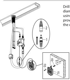
Drill a hole in the wall using a 6mm (1/4 in.) diamater drill bit. Install the battery pack (J1) using the molly anchor (J3) and screw (J2) provided. Insert the battery pack cable (1) into the control box connection (2).
