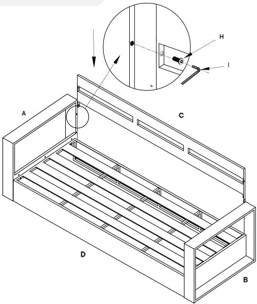
FULLY TIGHTEN ALL BOLTS TO COMPLETE THE ASSEMBLY.
