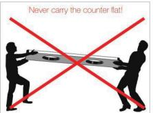
Remove counter from the box while maintaining it's vertical position. It is acceptable to use the sink openings as grasp locations, but highly preferable to also support it from the bottom. The vertical position must be maintained during the entire moving process.
