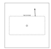
Outline tub on floor to ensure drain is centered
